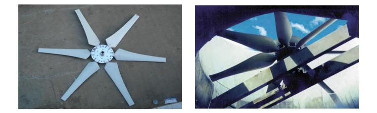
We are provided supply and services Aerodynamically designed adjustable blade type axial flow fan Is highly efficient ensure large air flow at low static pressure and low noise level
